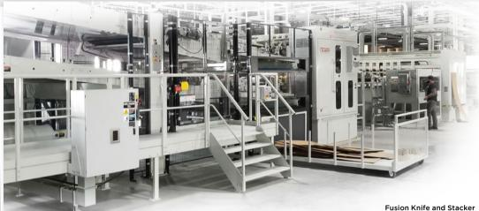
is standard, with an optional upstacker available. The downstacker features full-width transport belts. continuous radius transport conveyor for precise
