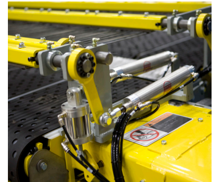
Spring Fingers or Brushes automatically adjust down-force to new order conditions
